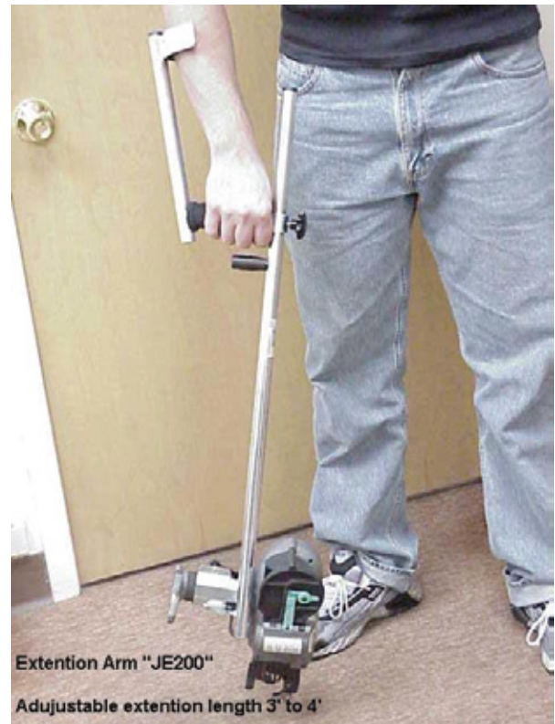
Figure 18: Extension handle on rebar tying machine. Courtesy of MAX USA Corporation ( www.maxusacorp.com , New York, USA)
