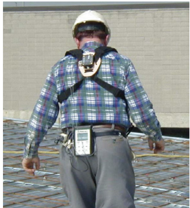
Figure 7: Rear view of the Gyroscope and DataLog II used to collect trunk posture.
