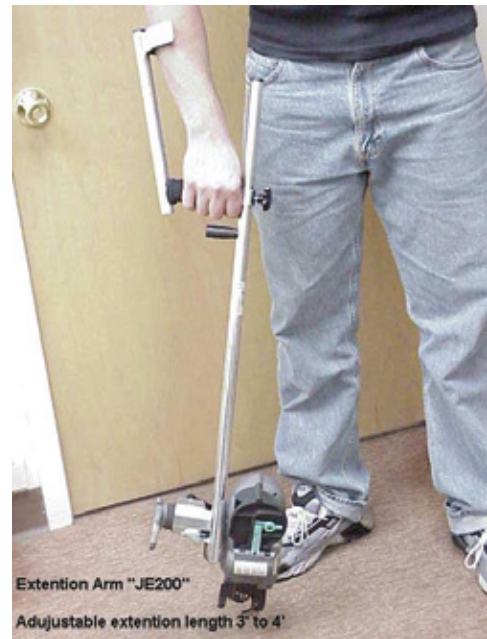
Figure 1: Rebar-tying machine with (left photo) and without extension arm (right photo).
