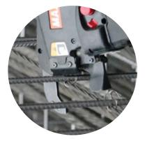
Rebar tying technology efficiently automates each tie to use as much wire needed for the specific rebar combination, which eliminates wasted material and saves on wire costs.
