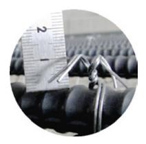
The MAX TwinTier's wire bendin mechanism creates a low profile tie that bends at the edges as opposed to the wide loop tie most rebar guns carry out that can pose a snagging hazard in the field.
