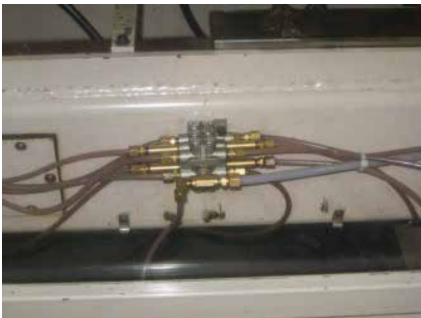
12-Port Distribution Block on Blow Molder
