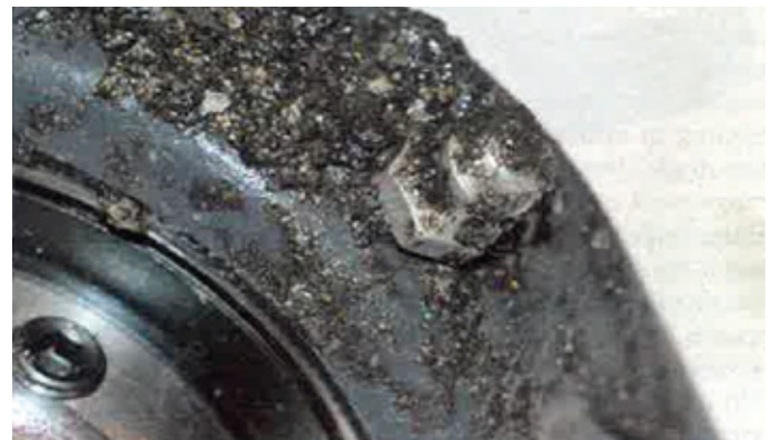
Figure 2: Before lubricating a bearing, make sure the grease fitting is clean so contamination is not introduced into the bearing during relubrication.
